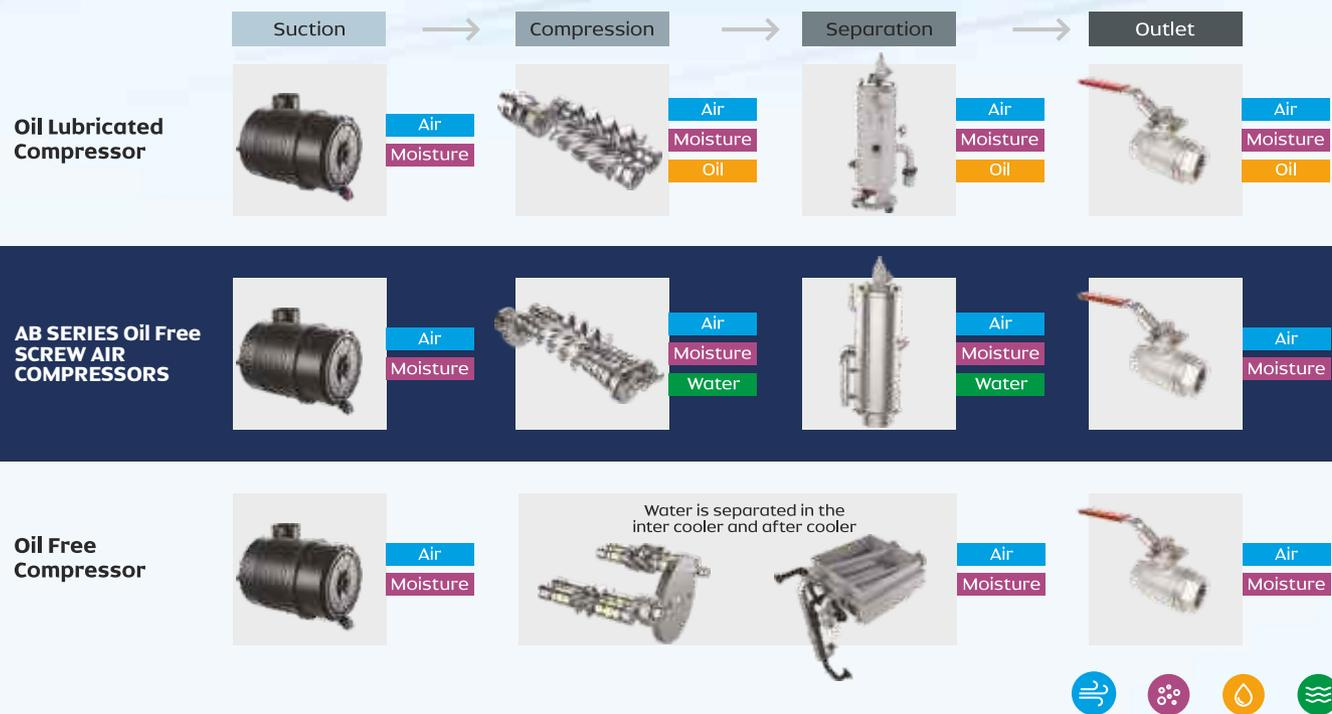
At ELGi, we've re-defined oil free compressor technology and built products that deliver high performance with minimal environmental impact. Today, our oil free compressors support some of the most critical and sensitive applications which demand, not just a high level of air quality, but also zero mineral oil residue.
